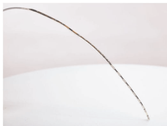
Figure 1. The Freedom-8A spinal cord stimulation neurostimulator with eight electrodes, a microchip, and a separate miniature receiver (not shown).
